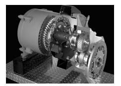
Durable components – Generac's gearboxes and elastomeric couplings are well proven designs. With thousands of gear driven gensets produced over the past 15 years, this system has demonstrated outstanding durability.
